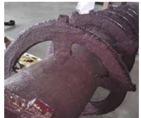
Screw Auger coated in Belzona 1811
